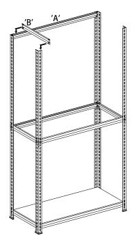
Fix Brackets 'A' at the very top allowing enough room for the MDF Shelf to sit against the legs. Repeat with Brackets 'B'.
