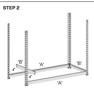
Use Shelf Brackets 'B' for the side brackets, using the Shelf Bracket from Step 1 as a guide for height. Allow one keyhole free from the ground as shown in the diagram. Use the same Shelving Brackets for opposing sides as shown in the diagram.
