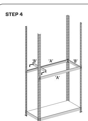
Fix brackets 'B' so that the top rivet sits on the upper legs and the bottom rivets sit on the lower legs. Repeat with brackets 'A'.
