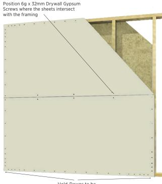
Hold-Downs to be positioned at each end of the USG Boral bracing element
