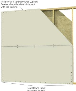
positioned at each end of the USG Boral bracing element
