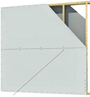
Position 6g x 32mm Drywall Gypsum Screws where the sheets intersect with the framing
