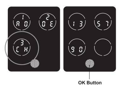
While in **Programming Mode**, select "3CH" to check registered **Access Codes**. If you are not in **Programming Mode**, please see **Section 3.2** to enter **Programming Mode**.
