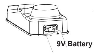
Your Lockly™ will automatically detect battery polarity. So hold your 9V battery lead in place against bottom of the Lockly™ to **temporarily** activate the screen to enter your **Access Code**. Be sure to hold the 9V battery against the contact points located at the bottom of the lock until you have successfully unlocked your door with your **Access Code**. Once unlocked, batteries should be replaced immediately.
