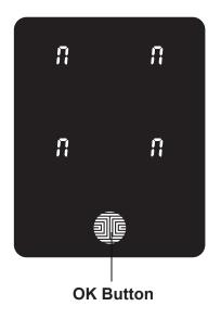
If the two (2) **Access Codes** you entered does not match, an error message will appear on the screen (As shown to the left). Press **OK** to return to the **Programming Screen** and try again. See **Section 3.3**
