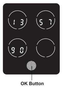
Active **Access Codes** will then be displayed on the screen in sequence from **left to right, top to bottom**. In the example shown on the left, the **Access Code** displayed is **1 3 5 7 9 0**.
