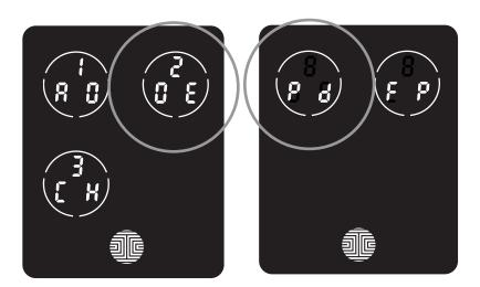
While in **Programming Mode**, select "**2DE**" to delete an **Access Code**. If you are not in **Programming Mode**, please see **Section 3.2** to enter **Programming Mode**.
