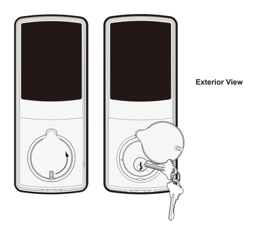
To **unlock** your Lockly<sup>™</sup> using the **physical key (supplied)**, open the key cover on the handle by turning the cover counter clockwise to reveal the **keyhole**.
