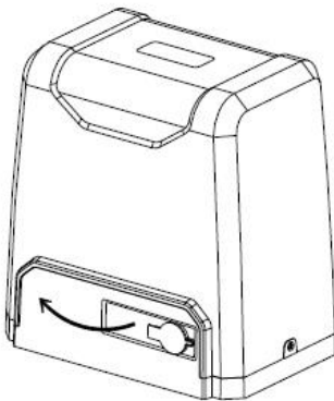
To put the gate motor into manual mode, insert the key and open the manual release bar as shown.
