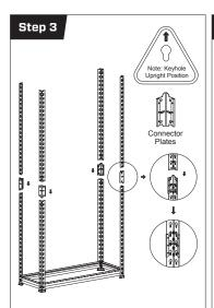
Place MDF shelf in bottom shelf to minimise buckling. Join the upper legs to the lower legs with the connector plates.
