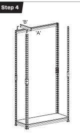
Fix brackets 'A' at the very top of legs 'C' allowing enough room for the MDF shelf to sit against the legs. Repeat with brackets 'B'.
