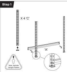
Place foot end caps onto the bottom of the legs 'C' (Note: Upright position). Place shelving bracket 'A' onto the legs 'C'. A rubber mallet can be used to lightly tap all brackets into the keyholes on the legs. Allow one keyhole free from the ground as shown in the diagram.
