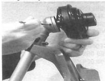
**1.** Consult Owner's Manual to determine method to lock shaft rotation (keyhole for interference fit or wrench to lock rotation of gear case).
