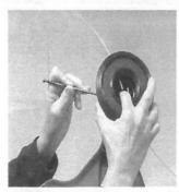
**5.** Hold nut or bolt in place with finger and secure tightly onto shaft by turning head while the shaft rotation is locked.
