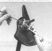
2. Locate keyhole and lock gear case.
