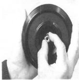
**4.** Place the identified nut or bolt into the recessed hex area of the SaberCut head.
