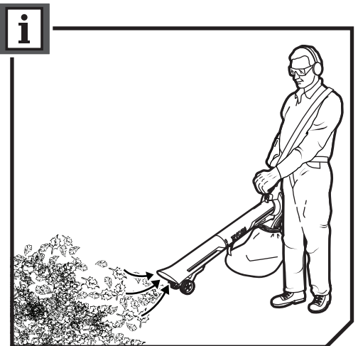
Hold the product by the designated handles and operate the product in the recommended position as shown. The wheels work best when used on a flat surface such as a concrete patio or sidewalk.
