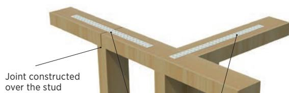
400 x 25 x 0.9mm galvanised connection strap. A 3 kN connection strap requires three 30 x 2.5mm galvanised nails on either side of the joint. A 6 kN connection strap requires six 30 x 2.5mm galvanised nails on either side of the joint.
