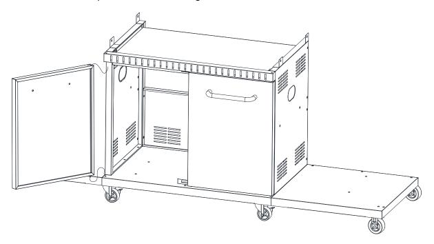
**Step 8:**Assemble the firebox (4) into the cabinet use bolt (A) 4pcs as shown.
