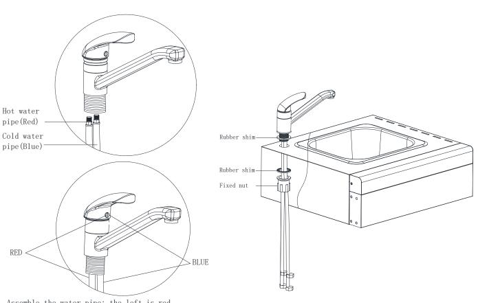
Assemble the water pipe: the left is red and the right is blue.
