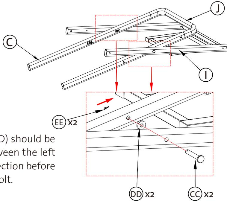
The washer (DD) should be located in between the left and right leg section before inserting the bolt.
