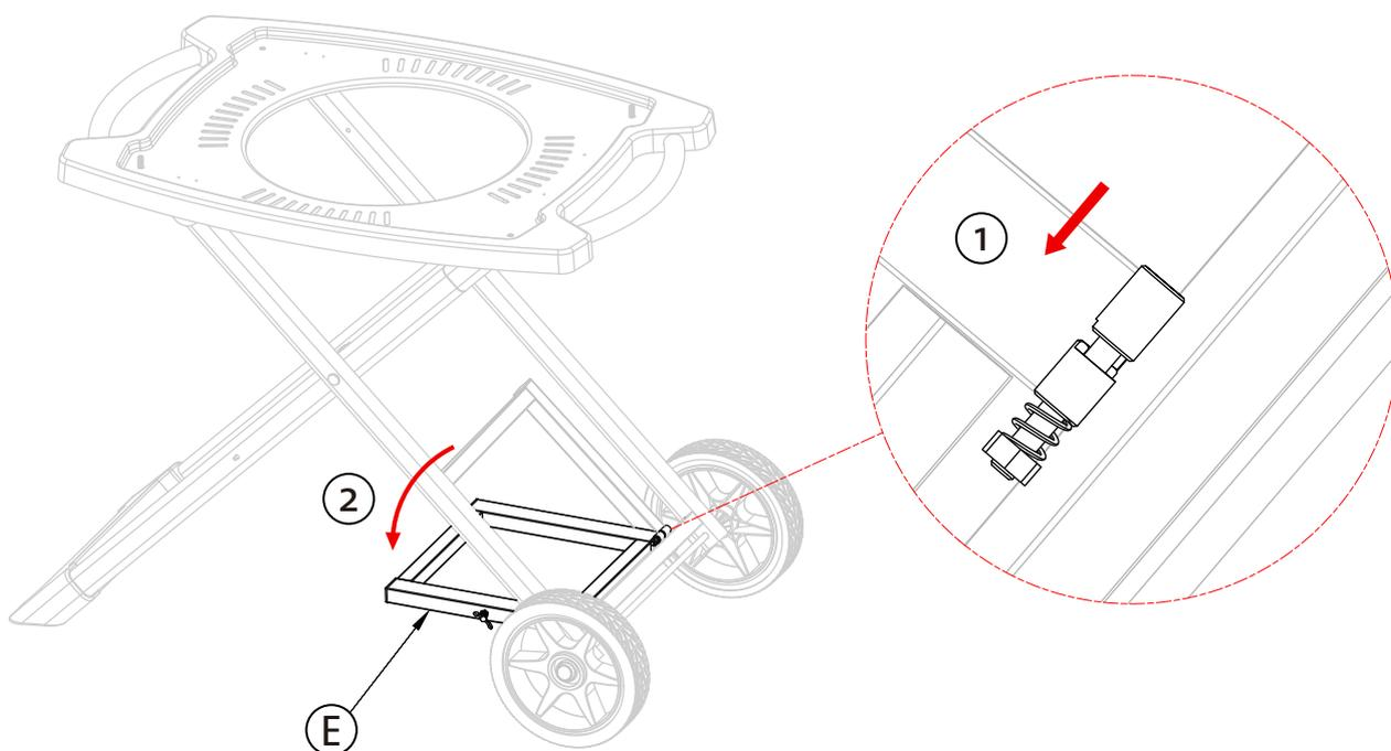
To fold up the gas cylinder mounting base (E), simply lift it up as shown below.
