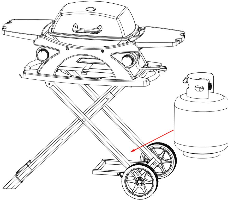
Use the wing nut on the side of the mounting base to tighten and secure the cylinder in place.
