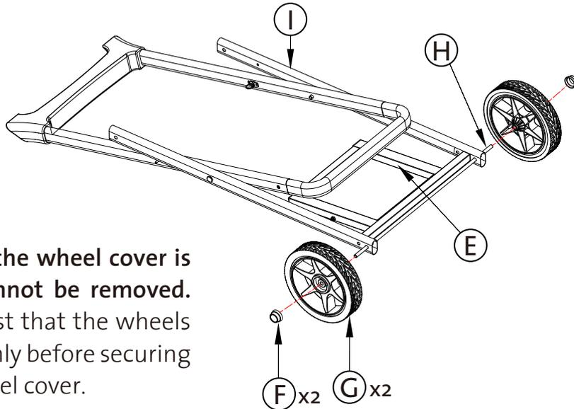
**NOTE: Once the wheel cover is secure, it cannot be removed.** Be sure to test that the wheels move smoothly before securing with the wheel cover.
