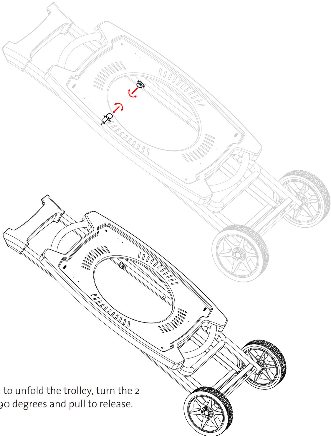
Note: to unfold the trolley, turn the 2 pins 90 degrees and pull to release.
