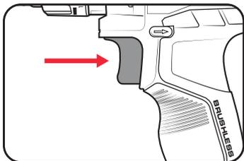
2. Check the forward/reverse lever is on the desired setting.
