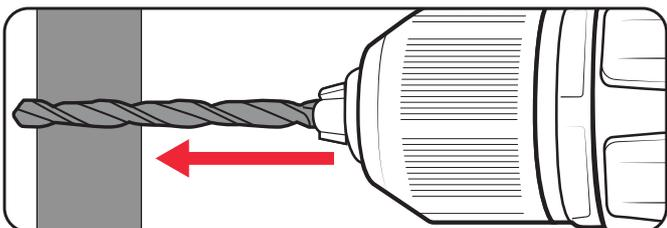
**Note:** Do not force the drill or apply side pressure to elongate the hole. Let the drill do all the work.
