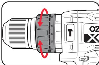
**Note:** Selecting a higher torque setting will allow the drill to use more torque to drive the screw in or out. To prevent damaging the screw head, it is recommended to start at a low torque setting and increase when necessary.
