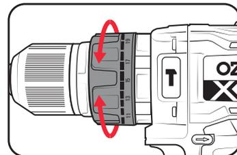
2. If the clutch ratchets and makes a clicking sound before screw is flush, increase the collar setting and continue tightening.
