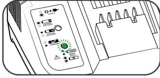
2. Align and then slide the ribs on the battery into the recess in the charger.
