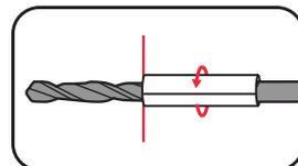
3. Drill into the material until the surface reaches the start of the tape.
