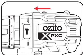
2. Adjust the torque by rotating the torque collar to the desired setting.
