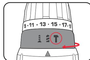
**Note:** 2nd gear (high speed) is recommended for hammer drilling.
