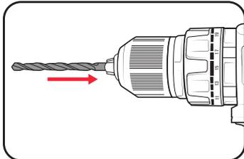
3. Tighten the chuck by turning the chuck collar clockwise.
