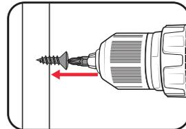
3. Repeat until you reach the correct setting/screw depth. Use this setting for the remaining screws.
