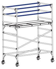
Add the last set of diagonal braces. Fit toe boards to all working platforms. Then position the 4m scaffold ladder, going through the hatch of the platform. Add the ladder support onto th 2nd rung of the 5-rung frame, as shown in the diagram below.
