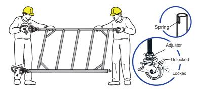
2. Position the ladder frame as shown. Lay it on a flat surface vertically and clip the horizontal braces and bottom brace onto the frame rung to square the scaffold unit.
