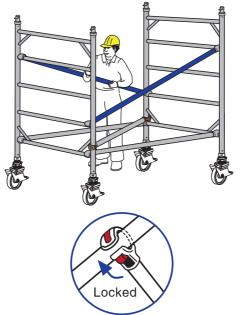
4. Locate the platform on the top rung of the 5-rung frame. Ensure that the scaffolding is correctly aligned by using a spirit level.
