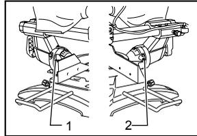
1. Right 5° bevel angle adjusting bolt
