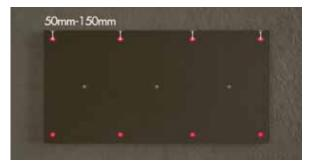
2. 4 No. fasteners along each length - no less than 50 mm - no more than 150 mm from edge of board, 3 No. fasteners along the middle (Offset from edge positions as per diagram).
