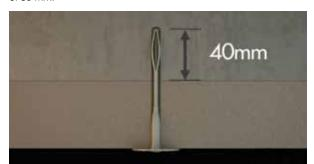
The fasteners should be evenly distributed over the whole area of the board and must offer a minimum 40 mm penetration into a solid substrate.
