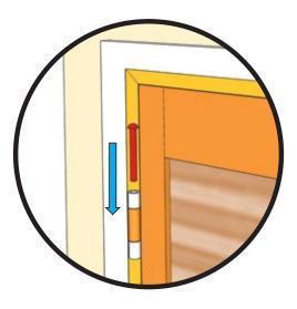
Once Frame is securely fitted to the window, the Panels can be installed one-by-one. The same process is used for both Recess and Face Mount applications.
