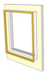
FACE MOUNT - Align constructed frame with window architrave. NOTE: Not all architraves are square, please check before installation.
