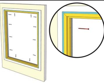
Once the matching packing pieces form a secure fit into the recess, ensure frame is square and fit into place using screws provided. Pre-drill as required.
