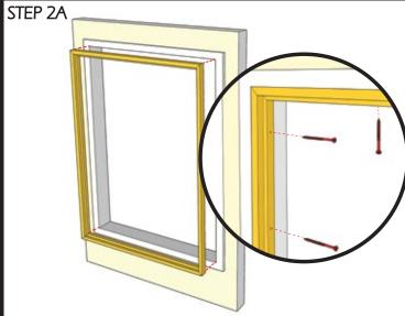
**RECESS MOUNT** - Align constructed frame with window and insert into opening. Ensure frame is square and fit into place using screws provided. Pre-drill as required.
