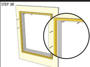
**FACE MOUNT** - Ensure frame is square and fit into place using screws provided all way around the frame. Pre-drill as required.
