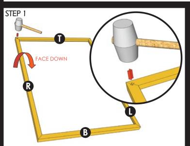
Identify Top/Bottom/Left/Right Frame lengths, lay face down on a soft flat surface. Use Hoffman Key and mallet, wedge into place forming strong corners
