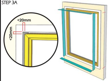
**RECESS MOUNT** - If the recess opening is slightly larger than the frame, 2.5mm and/or 5mm packing pieces can be used to fill up to 20mm in total width & height.
