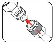
**WARNING!** Always use a coupling that discharges all the compressed air in the tool at the time the fitting or hose coupling is disconnected. Using a coupling that does not discharge the compressed air could cause unintended operation and serious personal injury.
