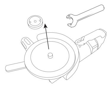
3. Hand tighten the Lock Nut using the supplied spanners in the opposite direction.
