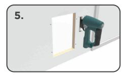
Using a reciprocating jigsaw, cut along marked lines.
