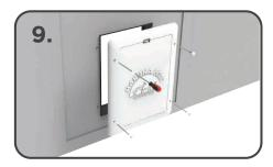
Screw into door from the inside. WARNING: Over tightening of screws will cause damage.
