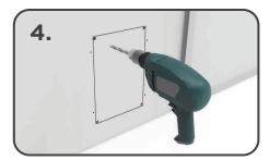
Drill a hole in each of the 4 inside corners with a minimum of 10mm drill bit.
