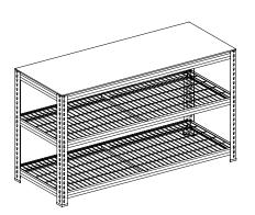
Lay Timber Bench Top 'E' between the top brackets as shown to complete your bench.
