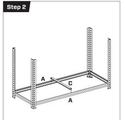
Slot Brace 'C' into position through the holes provided on Brackets 'A'.
