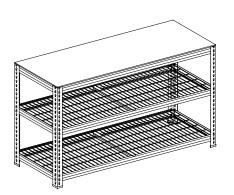
Lay Timber Bench Top 'E' between the top brackets as shown to complete your bench.
