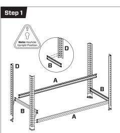
Add Foot End Caps to bottom of Legs 'D'. Fix Brackets 'A' to the bottom of Legs 'C' as shown followed by Brackets 'B'. A rubber mallet can be used to lightly tap all brackets into the keyholes of the legs. Allow one keyhole free between the foot end cap and the shelving bracket.
