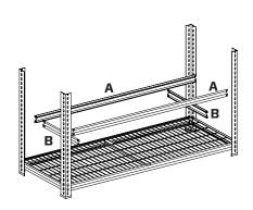
Lay Wire Shelf between the bottom brackets as shown. Fix Brackets 'A' and Brackets 'B' to desired shelf height. As before, a rubber mallet can be used to lightly tap all brackets into the keyholes of the legs. Slot Brace 'C' into position through the holes provided on Brackets 'A'.
