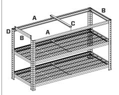
Lay Wire Shelf between the middle brackets as shown. Fix Brackets 'A' to the top of Legs 'D' as shown followed by Brackets 'B'. A rubber mallet can be used to lightly tap all brackets into the keyholes of the legs. Slot Brace 'C' into position through the holes provided on Brackets 'A'.
