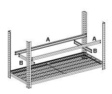
Lay Wire Shelf between the bottom brackets as shown. Fix Brackets 'A' and Brackets 'B' to desired shelf height. As before, a rubber mallet can be used to lightly tap all brackets into the keyholes of the legs. Slot Brace 'C' into position through the holes provided on Brackets 'A'.
