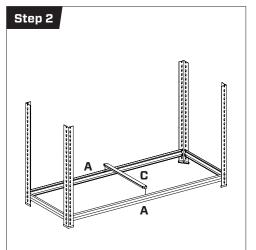
Slot Brace 'C' into position through the holes provided on Brackets 'A'.
