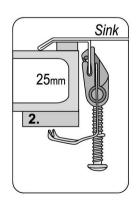
These anchor braces are designed for use with bench tops tops 30-40 mm thick (1). If your counter top is thinner, insert wooden wedges between the counter top and the braces so as to secure them (2). After placing two at each corner of the sink, place the rest evenly spaced around the perimeter of the sink.
