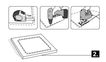
Draw another line 10 mm inside the first line. cut a hole in the bench top following this second, inner, line. (\*if the manufacturer has included a pattern in the package, then use the pattern to cut the hole in the bench top).
