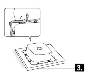
Adhere the rubber bench seal around the under side of the edge of the sink, being careful to lay it smoothly (without ridges).
