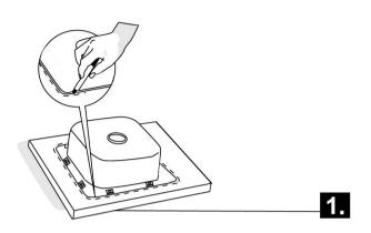
Place the sink upside down in the position where it is to be installed, and trace the outline of the sink on the bench top with a pencil.
