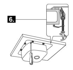
Tighten the screws of the anchor braces (with a hand screwdriver), to secure the sink in place.
