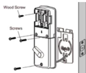
15. Connect the cable of the exterior unit to the interior unit, ensure the deadbolt tailpiece is engaged with the turn piece. Then align the interior unit and secure it with the screws. Insert 4 (AA) 1.5V batteries and slide the battery cover onto the interior unit.
