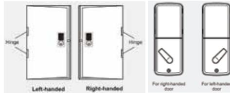
13. Face the door from the outside. The door is left-handed if the hinges are on the left side of the door, whereas the door is right-handed if the hinges are on the right side of the door. Rotate the thumb turn piece to the left at 45 degrees for right-handed doors. Rotate the thumb turn piece to the right at 45 degrees for left-handed doors.
