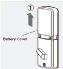
14. To remove the battery cover, push it up first, then pull it out.
