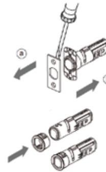
2. Determine which latch mounting method will be used (square plate or drive-in) and make the necessary adjustments. No adjustments are required for the square latch face plate.
