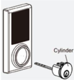
10. Install the cylinder into the deadbolt keypad with the tail piece in horizontal position inserted through the hub of the latch.
