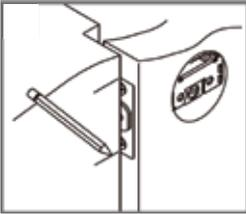
8. Close the door against the frame and mark the latch position for fitting of the striker.
