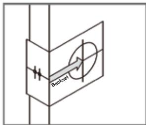
3. Establish the height and backset for the lock on the door.
