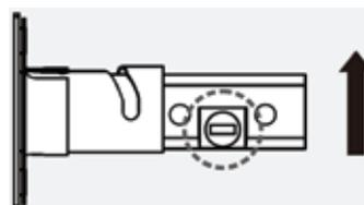
7. Remove any loose saw dust, insert the latch and secure it with the two wood screws provided. Make sure the cross is on the bottom of the latch. Please do not fully tighten the screws until the lock is completely installed. For the drive-in latch, drive the latch into the hole on the edge of the door.
