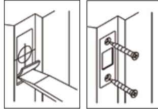
9. Measure one half of the door thickness from the door stop and vertically mark the centre line of the striker. Drill a 25mm (1") diameter hole, 25mm (1") deep at intersection of the horizontal and vertical lines. Chisel out a 2mm deep recess along the striker outline to allow the striker to sit flush against the doorframe. Secure the striker with the wood screws provided.
