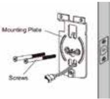
12. Pass the IC wire through the wire hole of the mounting plate on the interior side of the door. Fix the mounting plate with screws onto the door face. Make sure the deadbolt keypad on the outside is straight.
