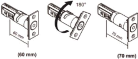
1. Adjust the latch to the desired backset (60mm or 70mm). Backset is the distance from the door edge to the centre of the hole on the door face. To adjust the latch to the 70mm backset, rotate the latch until it stops. Reverse the direction to return to the 60mm backset.
