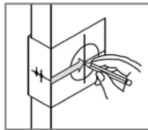
4. Use the template provided as an indication to mark the centre of the circle on the door face and the centre of the door edge.
