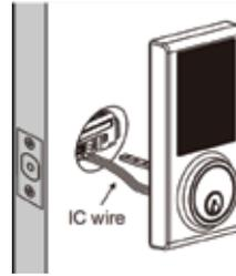
11. Pass the IC wire under the latch to the interior side of the door and insert the tail piece through the cross-shaped crank of the latch.
