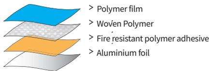
Ametalin utilises Advanced Laminating Technology; the polymer adhesive remains tacky indefinitely and provides superior resistance to heat, fire and delamination.
