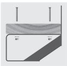
3 Install each timber tread using M8 x 60 mm cup head bolts, nuts and washers.
