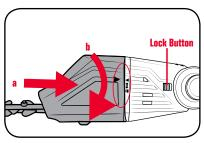
**Note:** The Lock Button will "CLICK" back to the left (original position) when the trimmer head is correctly secured in place.
