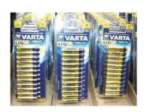
Blister packs made to size with recyclable materials allow the product to be visible to the customer but prevent it from being removed or damaged in store.
