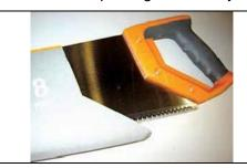
Place a cover over blades to prevent contact with sharp edges.
