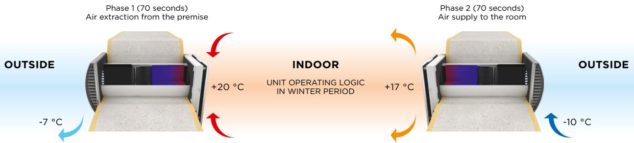
Warm stale air is extracted from the premise, flows through the ceramic regenerator and transfers its heat energy and moisture to it.
