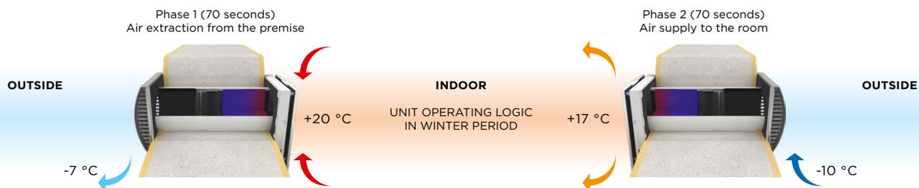
Warm stale air is extracted from the premise, flows through the ceramic heat exchanger and transfers its heat and moisture to it.
