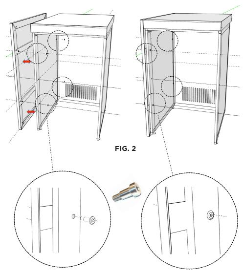
Align, Insert and Tighten the Barrel Bolts with the Alen key Provided.
