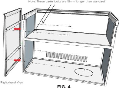
Note: These barrel bolts are 15mm longer than standard.
