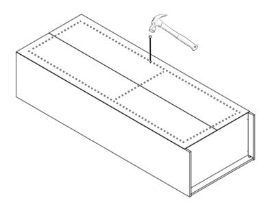
**Step 5:** Fold out the Backing Boards (7) proceed to nail the Backing Board into position with a hammer.
