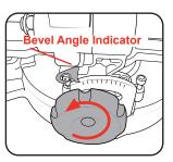
Tilt the cutting head to the desired bevel angle as shown by the bevel angle indicator.
