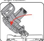
3. Tighten bevel lock knob at selected angle
