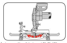
**Note:** The mitre table features positive click stops at  $0^{\circ}$ ,  $5^{\circ}$ ,  $10^{\circ}$ ,  $15^{\circ}$ ,  $22.5^{\circ}$ ,  $30^{\circ}$ ,  $35^{\circ}$ ,  $40^{\circ}$  and  $45^{\circ}$  for quick setting of common mitre angles.
