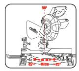
A bevel cut involves using a bevel angle other than 0° tilting saw to the left
