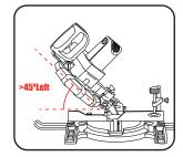
A compound mitre cut involves using a mitre angle and a bevel angle at the same time.
