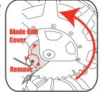
Depress the spindle lock button. To ensure it engages correctly, rotate the 6mm hex key until the spindle lock clicks into position.
