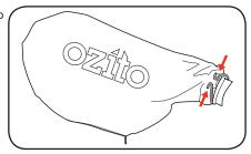
2 Slide the end of the dust bag over the dust extraction port and release the clamp.
