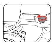
Rotate the mitre table to the desired angle using the mitre angle scale.
