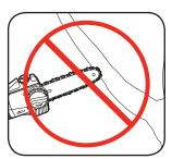
Do not saw with the tip of the guide bar. This could lead to kick back and possible injury.
