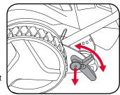
2. Release height adjustment knob and check that it is securely seated in the required cutting height position.
