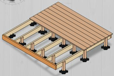
Starting from one side of the deck, attach the first decking board so it's flush to the edge of the deck. The decking board will overhang the first floor joist closest to the existing structure. Leave a 3mm to 6mm (0.125 - 0.25 inch) gap between the end of the decking board and the edge of the structure. Next, secure the remaining decking boards as per manufacturers instructions.
