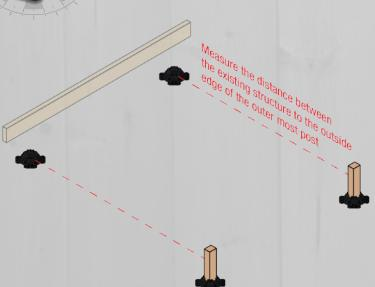
If building off an existing structure, measure from the structure to the outside edge of the post. (For example: If the deck will be 3 metres / 10 feet deep, position the block so that the outside edge of the post is 3 metres / 10 feet from the structure.) Do NOT use the the first row of blocks as a measuring reference. Use the same width between the TuffBlock piers as the first row.
