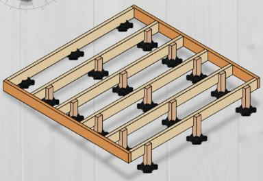
Cut posts to length and position them between the floor joist and the TuffBlock pier. Repeat this step until all posts are cut and positioned. Next, secure all floor joists and posts using two 75mm (3 inches) counter sunk batten screws.
