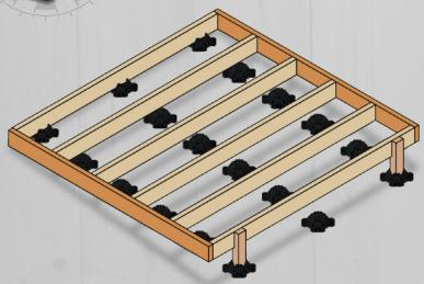
Using the frame as a guide, position the remaining TuffBlock piers directly beneath the frame. The blocks on the perimeter of the deck should be 300mm (12 inches) in from each end.
