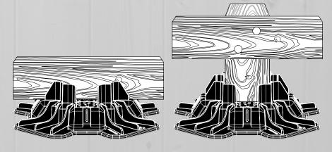
TuffBlocks are not designed for use in structures elevated more than 1 metre (39 inches) from the ground and should be installed on stable ground (see www.buildtuff.com for more details). As always, it is recommended to check your local building guidelines before starting any construction - we always suggest you get the thumbs up before starting your project.
