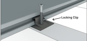
Ensure you have installed 1 (one) Locking Clip per board. Failing to install a Locking Clip will allow your boards to shift and come out of alignment.
