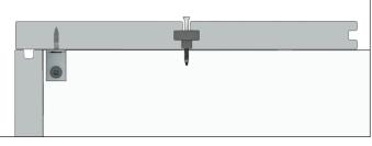
3. Repeat these steps and lay approximately 6-10 boards before screwing down properly (this is a guide only). Measure out from the 1st board to the last board to ensure that the boards are square.
