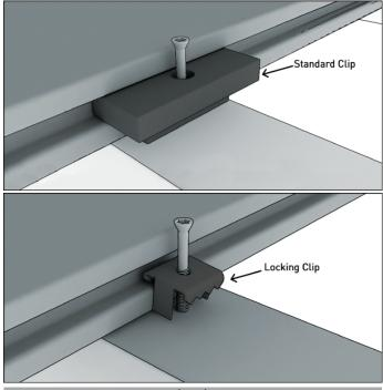
Ensure you have installed 1 (one) Locking Clip per board. Failing to install a Locking Clip will allow your boards to shift and come out of alignment.
