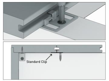
3. Gently push the next Ekodeck+ board into the clips, you may need to use a rubber mallet to seat the boards firmly in the clips.
