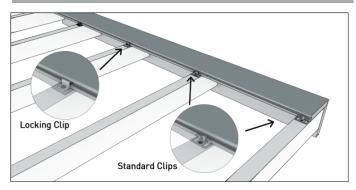
2. Screw down the clips ensuring they are tight and secure. You only need one screw per clip.
