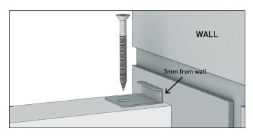
2. Run a string or chalk line from the front edge of the C-Clip between the first and last C-Clip and mark the remaining joists.
