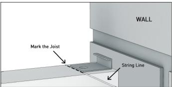
3. With the top of the joists now marked, install the rest of the C-Clips. C-Clips can be placed on every second joist if necessary. Gently push the first Ekodeck+ board into the C-Clips. You may need to angle the board slightly to push into the C-Clips.
