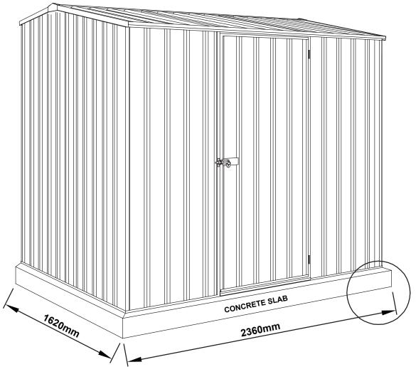
For construction in non-cyclonic areas Wind rating: N2 as per AS4055-2012
